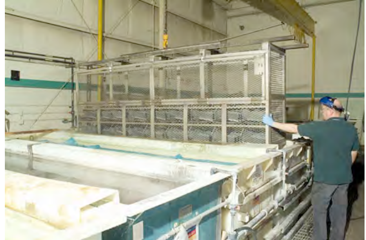
Seven-stage Pretreatment System for Iron and Zinc Phosphate that meets TT-C-490. System includes inline passivation and rust removal capabilities
